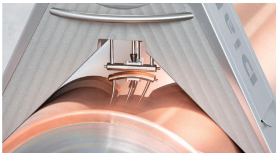
Tangential scanning with measuring bar
