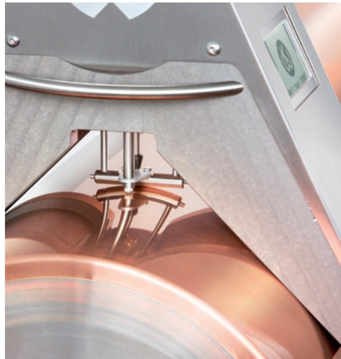
Temperature sensor and measuring bar
