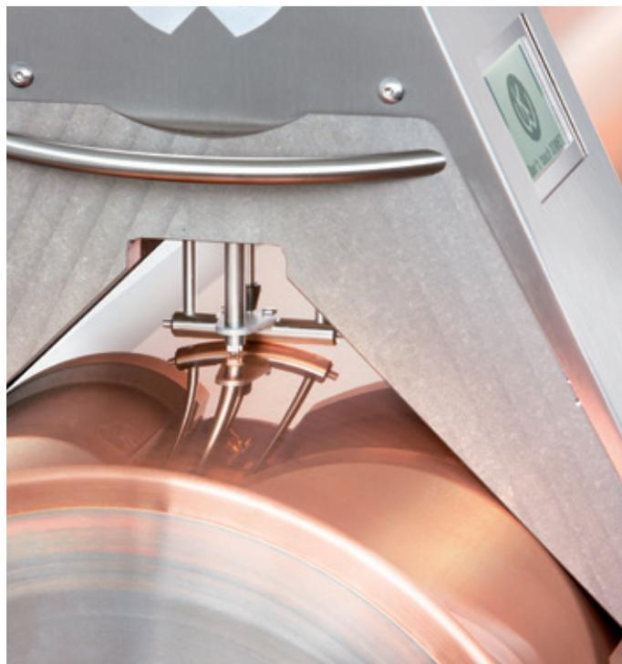
Temperature sensor and measuring bar
